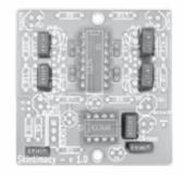
There are five different types of resistors. Don't worry about the orientation. It makes sense, though, to have parts of the same group facing the same direction.
